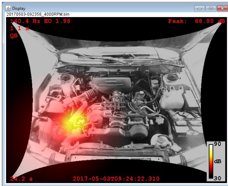
Automobile engine at 4304.6 RPM, engine order 2 (140.4 Hz).
