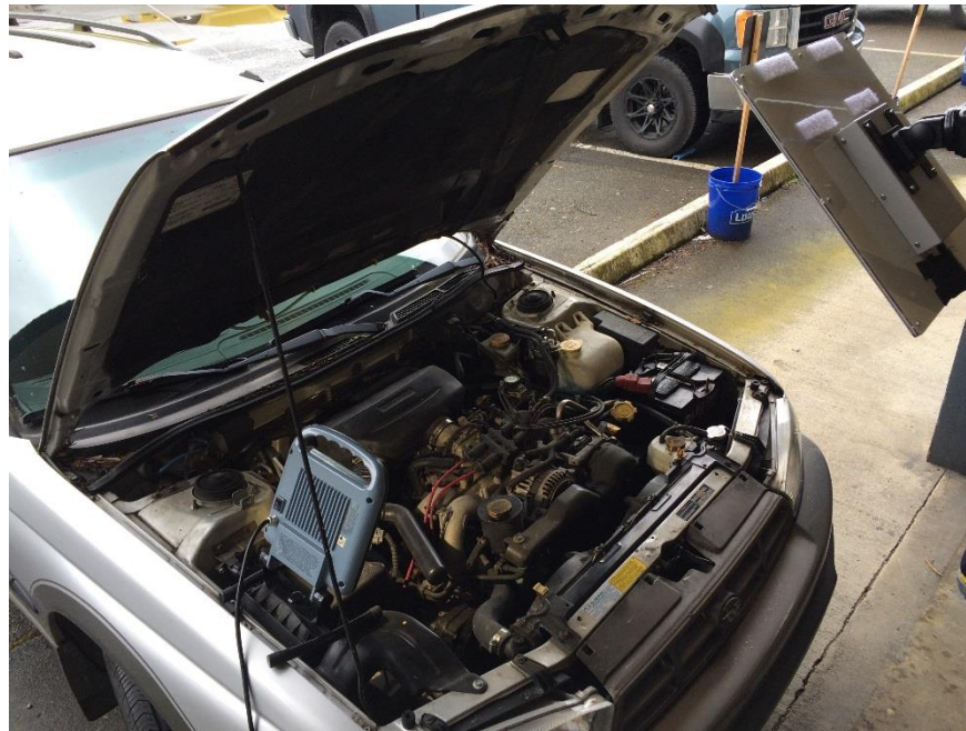
Setup for automobile engine order test.
